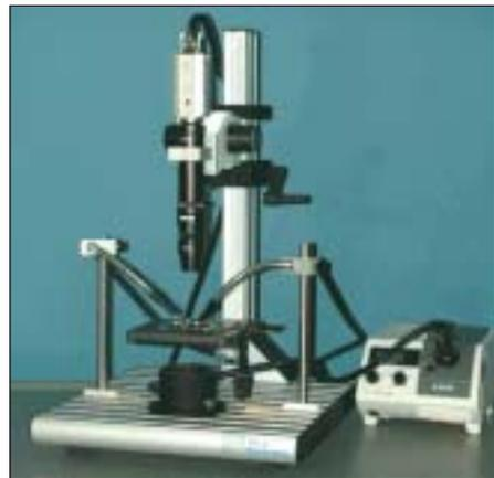
Manual X, Y stage adapted for a Navitar® zoom on a Tech Systèmes® bench.
