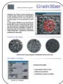
GrainSizer provides a rapid estimate of grain index according to the ASTM E-112 and NF04-102 standards.
