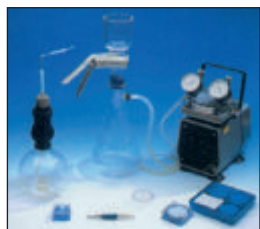
Membrane filtration system
