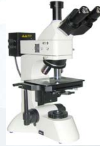
GXML3230BD RESEARCH Reflected & Transmitted Light (darkfield reflected) for Materials
